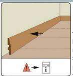
Note: If you must remove a board that has already been installed, slide it out horizontally to disengage the butt joint (see Figure 06). Do not lift it - this will damage the joint lock.
